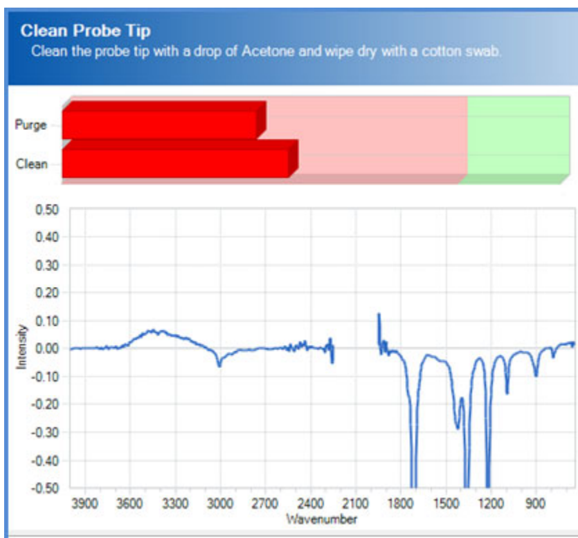
Figure 5-10 'Dirty' sensor—Poor cleaning method and subsequent collection of new background
