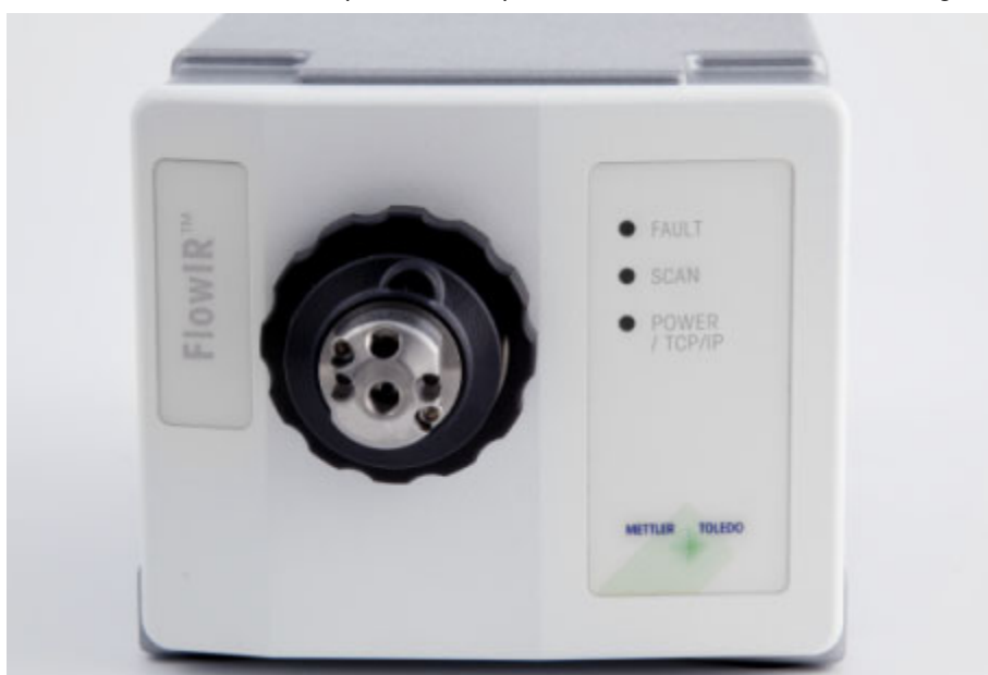
Figure 2-3 FlowIR base unit with non-heated flow cell head
