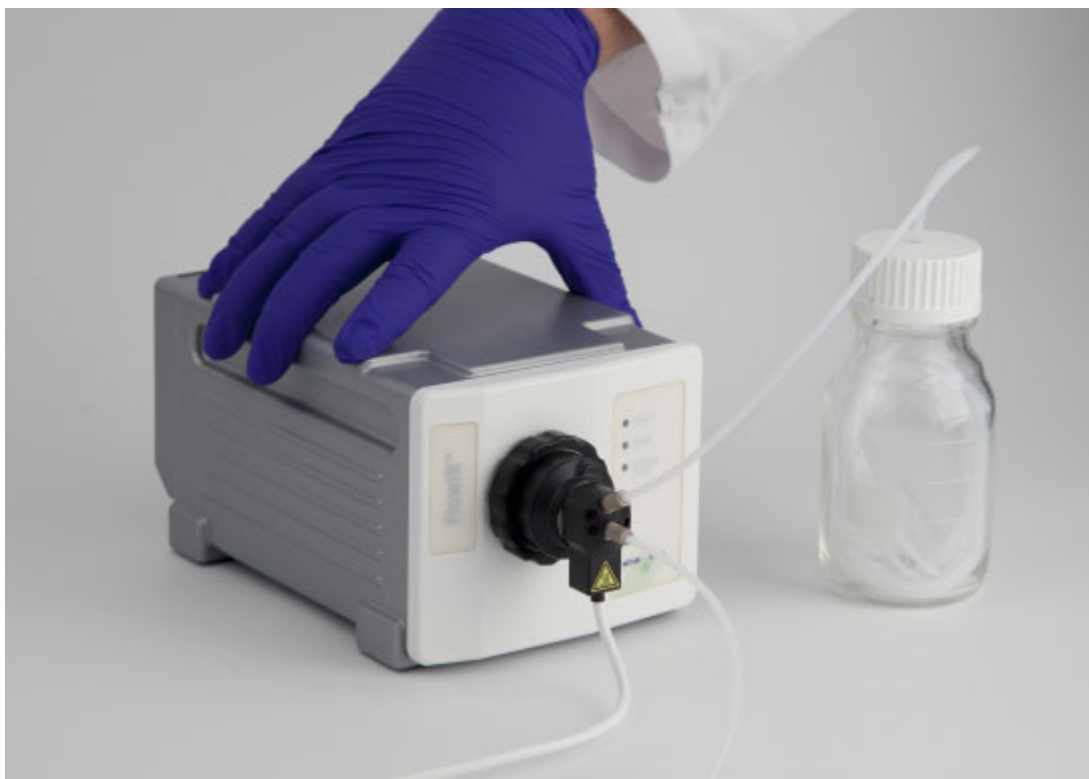
Figure 2-1 FlowIR—Base unit with sensor and heated flow cell head
