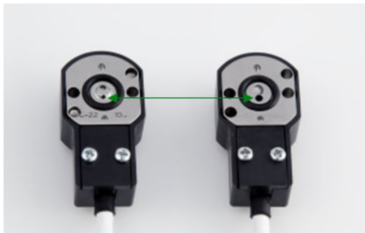
Figure 2-5 FlowIR volume heads—10 \mu L (left) and 50 \mu L (right)
