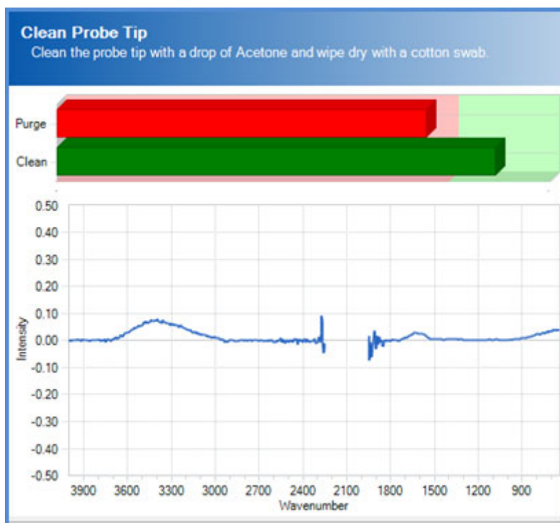
Figure 5-9 'Dirty' sensor—Prior reaction mixture or insufficient drying time of cleaning solvent
